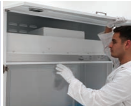
Top component fits filter/blower or can be used as storage
