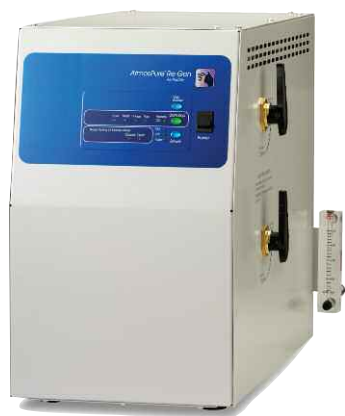
Photo 2: This gas purifier circulates the established inert atmosphere through a copper catalyst and molecular sieve to achieve oxygen and moisture levels below 1 ppm. It requires regeneration as little as once every one to three months so accommodates long-term experiments requiring oxygen and moisture levels as low as 1 ppm.
