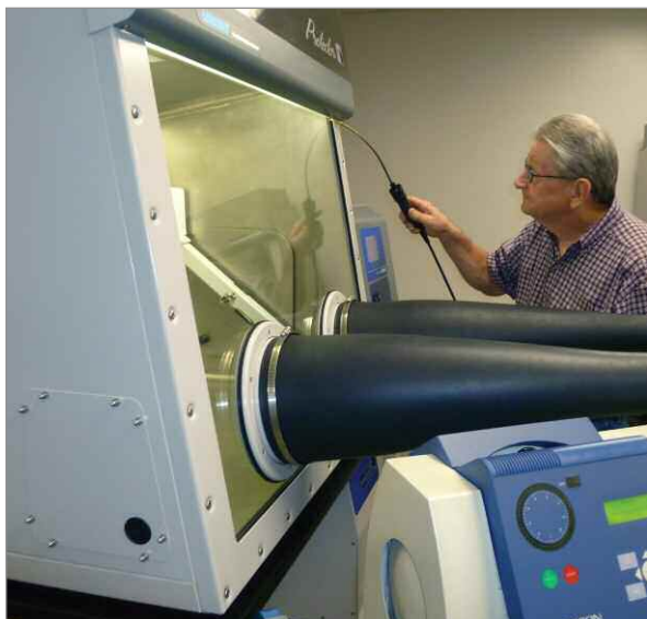
Photo 1: Tracer gas tests on the glovebox showed no detectable leaks greater than 1 \times 10^{-6} ml/second, which calculates to less than 0.09 ml per day.
