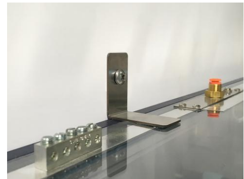
Correct Orientation of Wall Bracket On Top of the Desiccator
