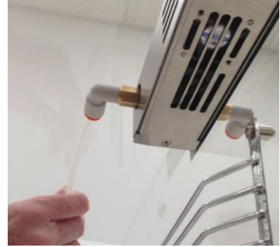
Photos 10, 11: Push 0.25" tubing into the gas fittings on the Smart RH module from the outside and inside of the desiccator.
