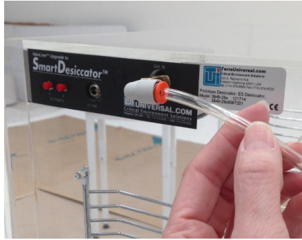
Photos 10, 11: Push 0.25" tubing into the gas fittings on the Smart RH module from the outside and inside of the desiccator.
