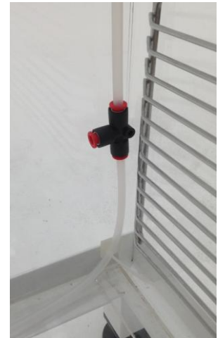
Photos 14, 15: T-connector on right-hand side of cabinet allows gas to be released and tubing to continue routing to the chamber's left-hand side, where it terminates
