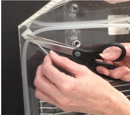
Photo 13: Reach inside the desiccator to trim the plastic tie after attaching tubing to adhesive loops
