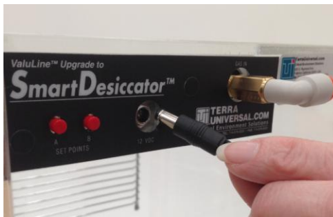
Photo 16: Electrical power connection
