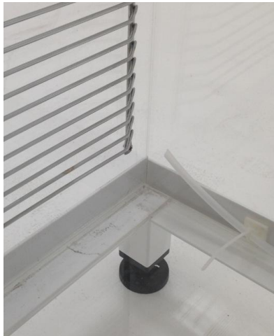
Photos 14, 15: T-connector on right-hand side of cabinet allows gas to be released and tubing to continue routing to the chamber's left-hand side, where it terminates
