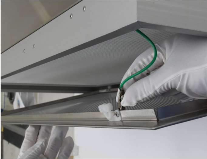
Photo 2: Remove grounding clip from the steel rivet post on the back side of the outer filter screen.
