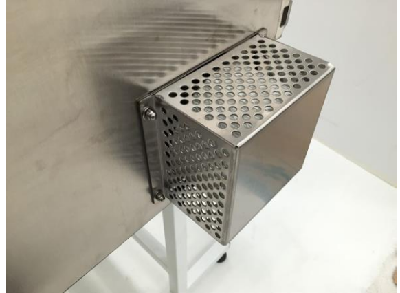
Figure 12: ULPA Filter Housing
