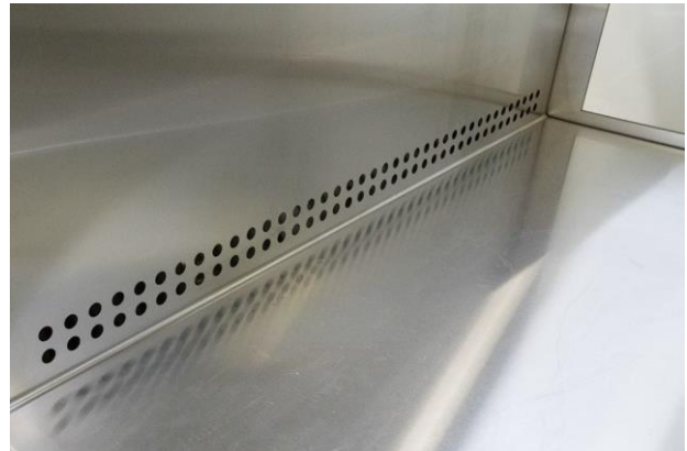
Figure 16: Air escapes through the exhaust vents along the bottom of the chamber
