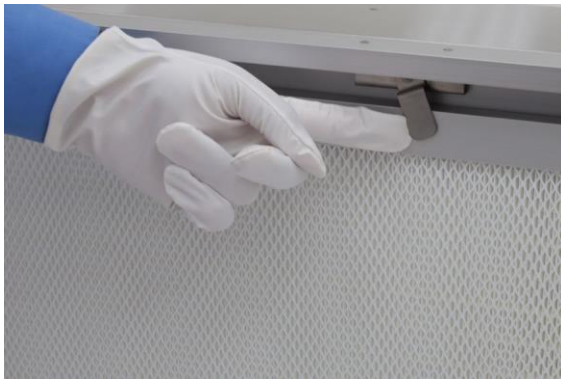
Figure 18: Rotate the retaining clips to release the filter
