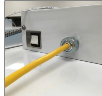
Figure 6: Cord grip on fan/filter unit housing
