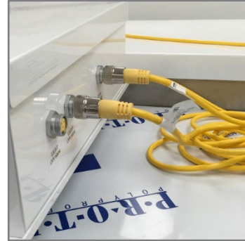
Figure 4: PDM connection for light fixtures
