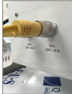
Figure 5: PDM connections for the fan/filter units
