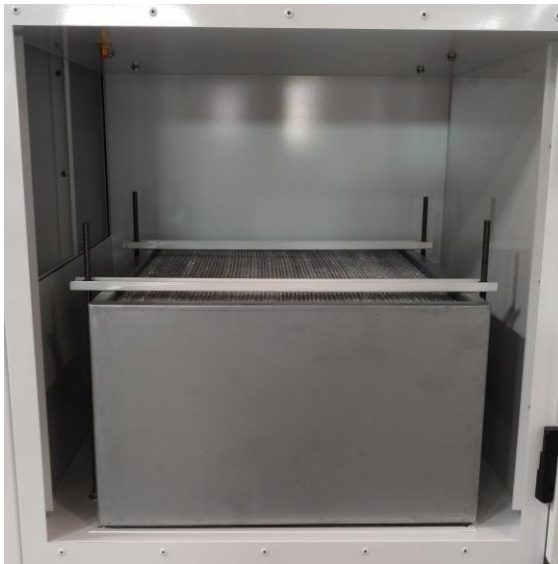
Figure 6: HEPA filter shown installed
