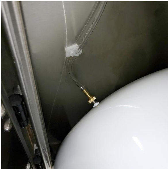
Figure 8. The port for the air pressure gauge can be found on the round end of the clean water tank
