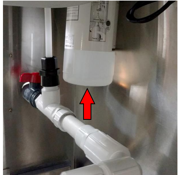
Figure 7. The soap dispenser reservoir can be found near the Fill Valve on the right-hand side of the cabinet.
