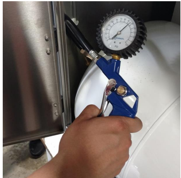
Figure 9. Disconnect the gauge line and use a flexible hose to connect an air compressor to the port for adjustment
