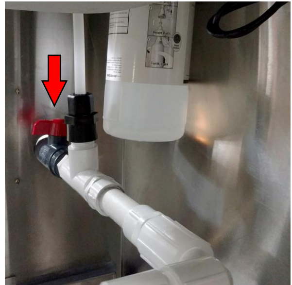
Figure 4. Open the fill valve to begin filling the tank
