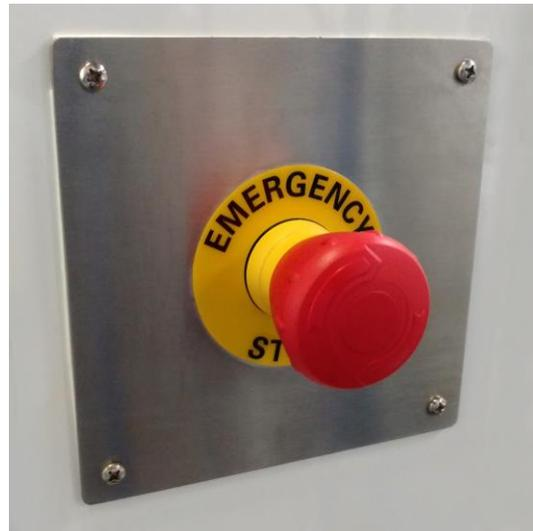
Figure 2. Emergency Stop Button (twist to reset)
