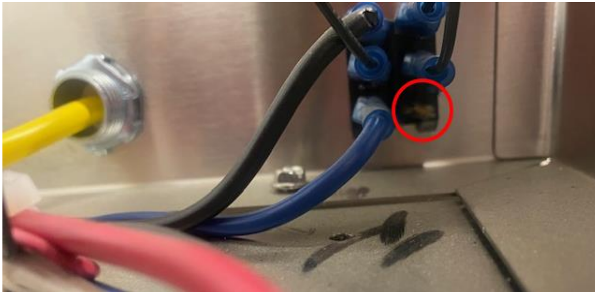
Figure 23. Take red cable and insert into empty slot on connector
