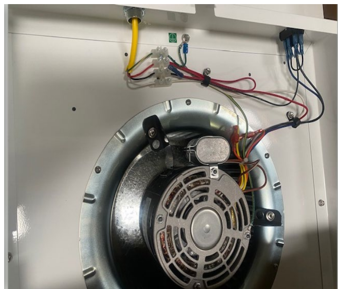
Figure 22. Red wire comes disconnected
