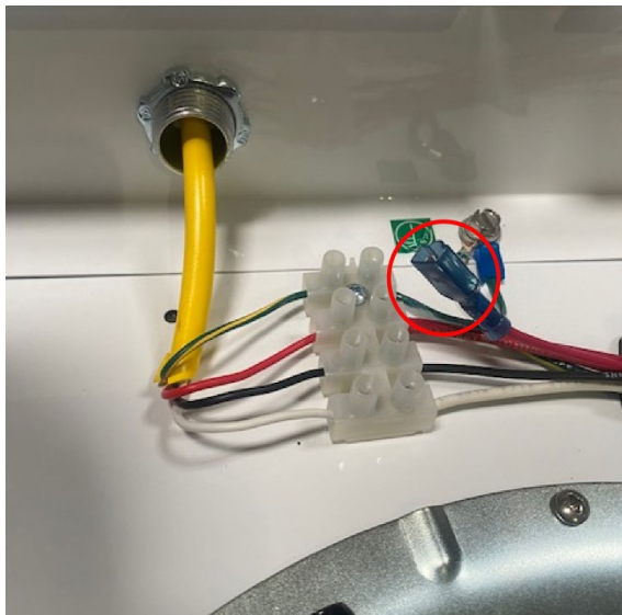
Figure 22. Red wire comes disconnected
