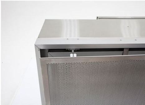
Figure 18: Friction catches hold the screen to the fan module housing
