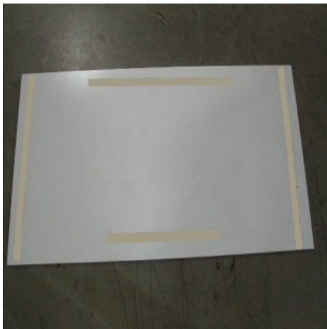
Figure 11: Polypropylene panel with tape
