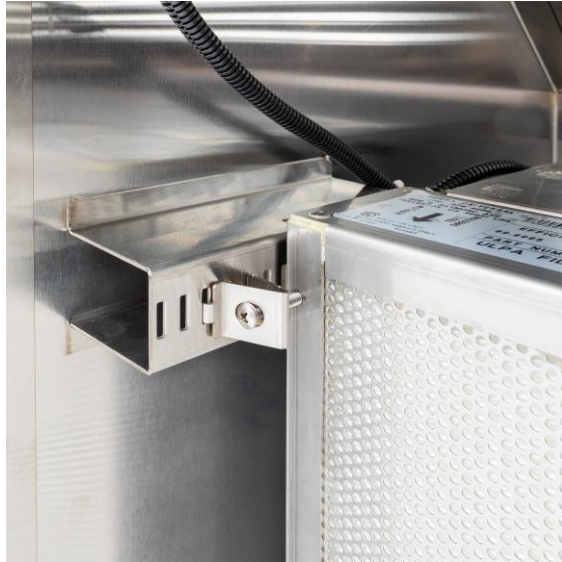
Figure 20: Rear panel clip detail — release clips to remove panel
