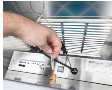
Figure 25: Challenge port — verify connections before power-on
