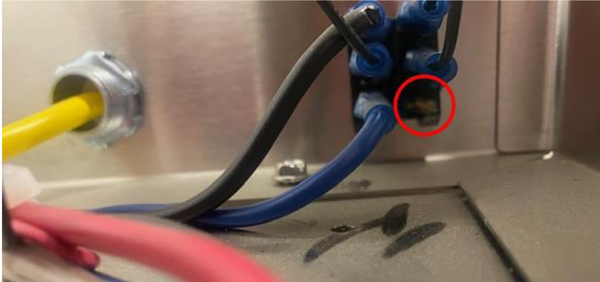
Figure 29: Take red cable and insert into empty slot on connector
