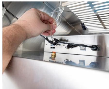
Figure 22: Filter track — ready for new filter
