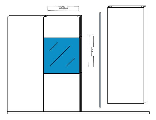
Once window panels are plumb and level, standard wall panel construction can be resumed
