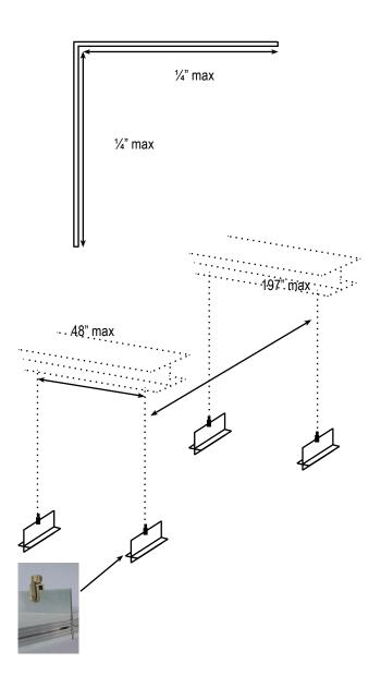
Ceiling panels should start to be fitted before the wall panels reach a maximum span of 1/4" to provide added structural stability
