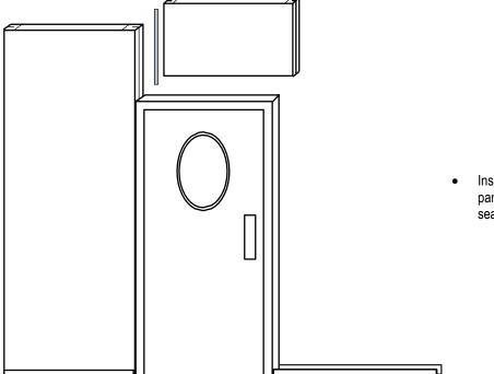
Insert aluminum tongue into adjacent panel and fit header panel in place, sealing as required
