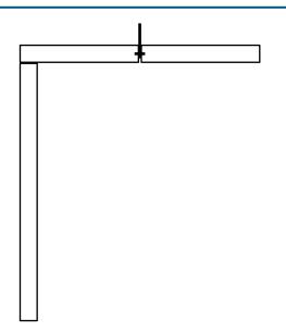
Ceiling panels should be placed on top of the wall panels or fitted to wall angles as defined by the specification and fit into the suspended hanging plates at panel intersections, and additional support points as required by the specification
