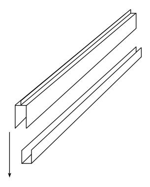
Place the top section of the recess base onto the bottom channel section
