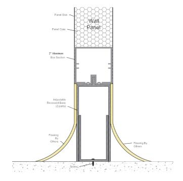
The panels are located onto base section using the inbuilt bottom edge box section in the panels. Once located, the panels can be sealed to the base section if required by the specification.
