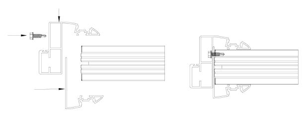
After fixing the U frame into the wall panels, add the panel union to the wall panels over the U frame, and slide the door header panel to complete
