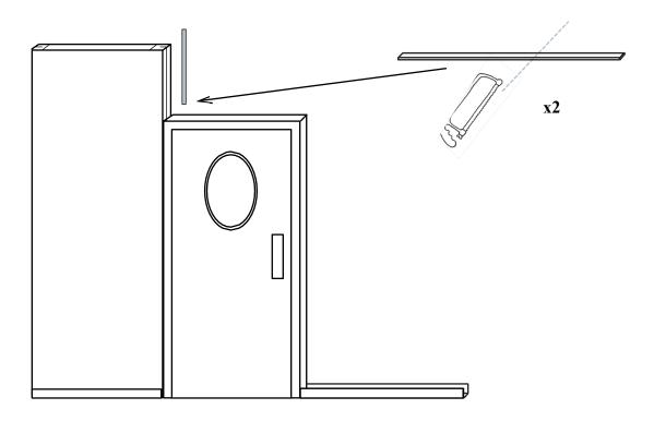
• Cut 2 lengths of aluminum tongue to fit above the door frame to which the header panel will be fixed
