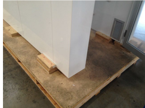
Photo 4: Air Tunnel shown on shipping pallet in between grooves created by wood blocks
