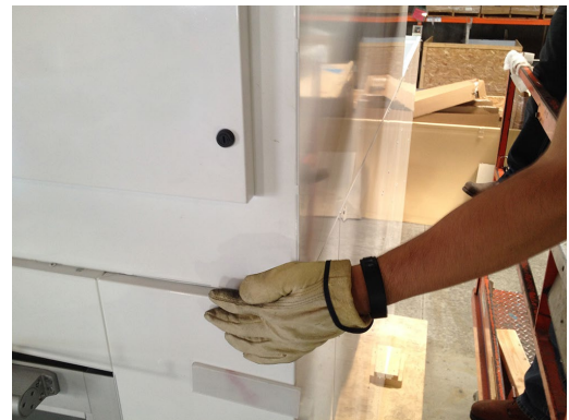
Photo 16: Blower Module shown manually pushed into place
