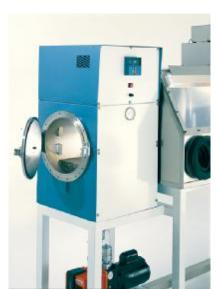
NOTE: It may be necessary to shim the hinge lugs on the door, depending on the thickness of the box material, in order for the spring-loaded hinge block to function.
