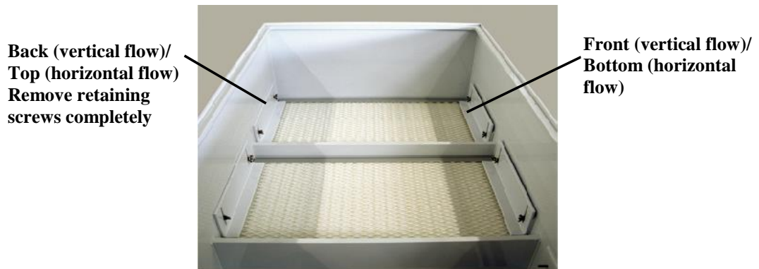
Replacing Filters Vertical flow model, shown with blower panel removed.
