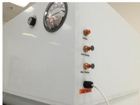
**Photo 2:** (From left) FFU control knob, Magnehelic™ differential pressure gauge, and certifier test ports
