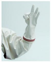
The Hypalon sleeve should be replaced every 6 months or if tears/holes are discovered upon inspection. Sleeve replacement should be performed immediately prior to the Daily Cleaning Procedure.
