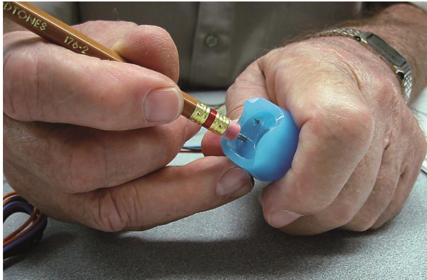
Figure 6: Use a pencil eraser to push the emitters out of the nozzle
