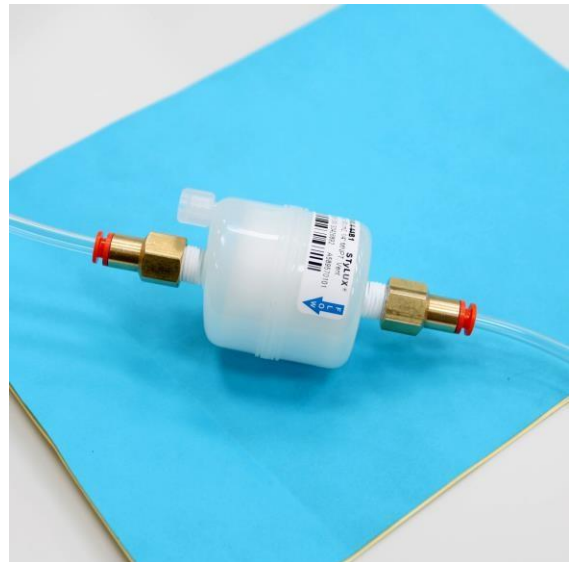
Figure 3: Assembled in-line filter capsule (notice the blue arrow indicating direction of gas flow)
