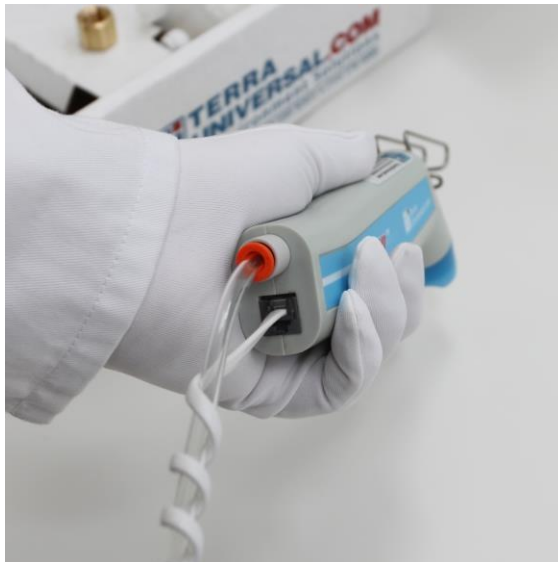
Figure 2: Gas and power connections at the base of the ionizing gun
