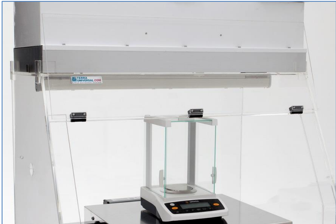
Figure 3: Place the IonBar™ on the hood frame before lowering the fan/filter unit into position.
