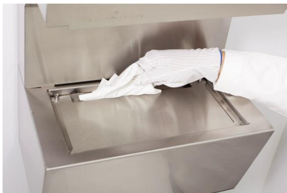
Wipe the rear air inlet cut-out with disinfectant
