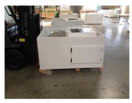
**Photo 8:** Forklift shown elevating the Blower Module with the 2"x4" wood stud centered underneath the unit as support
