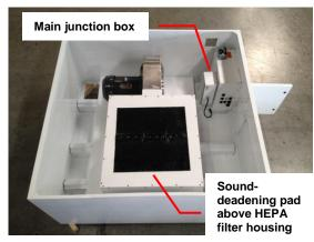
**Photo 7:** Blower Module shown placed on top of four (4) 2"x4" wood blocks, one (1) at each corner
