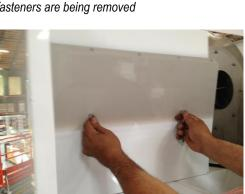
Photo 28: Inside panel door shown being removed
