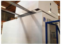
**Photo 14:** Forklift shown levering the Blower Module to enable removal of the 2"x4" wood blocks
