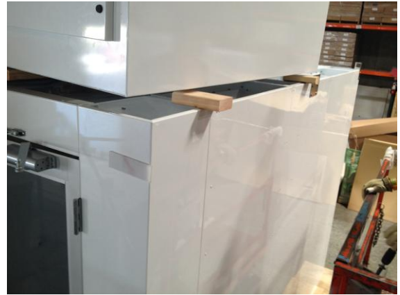
Photo 10: Blower Module shown positioned on the 2"x4" wood blocks at two (2) of the corners
