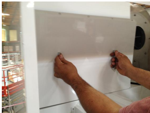
Photo 28: Inside panel door shown being removed
