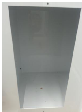
Photo 3: Vent removed. Pre-drilled hole shown for mounting to pallet or anchoring into the floor
