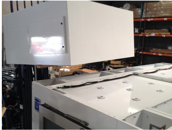
Photo 9: Blower Module being lowered onto the Main Enclosure in the correct orientation (electrical box shown)
