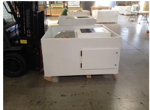
Photo 8: Forklift shown elevating the Blower Module with the 2"x4" wood stud centered underneath the unit as support
