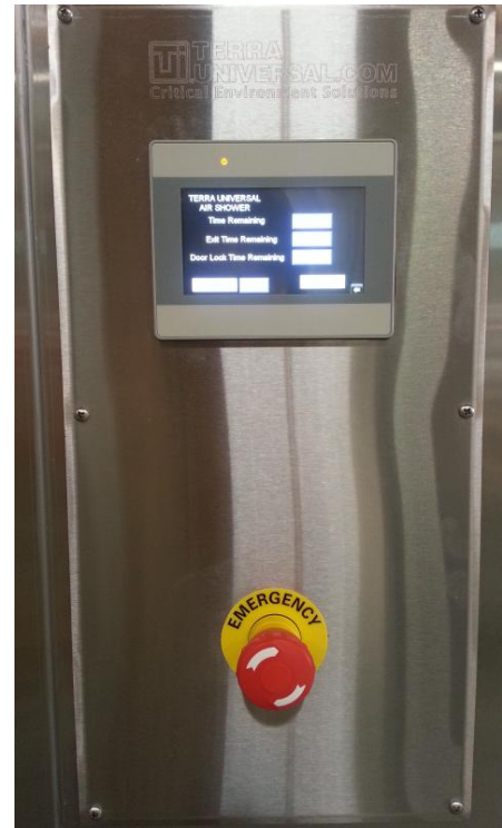
Photo 18: Touch Screen Control Panel
