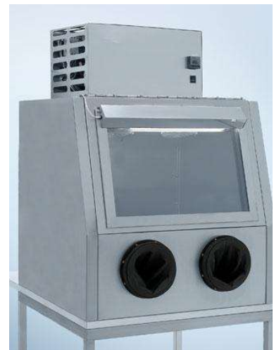
Figure 1. Partial-view window design with 10" glove ports and Constant Temperature Control system mounted above Glove Box
