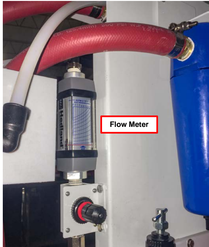
Figure 5. Flow Meter and Adjustment Knob
