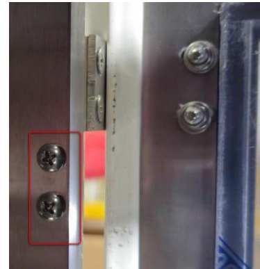
Figure 7.3: Remove screws inside passthrough to remove hinges
