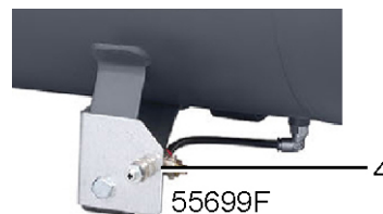
Figure 67: Drain valve of air receiver
