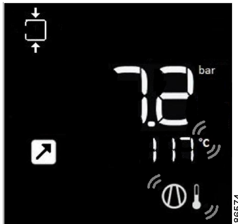
Figure 21: Main screen with temperature outlet shutdown
