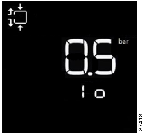
Figure 32: Indirect stop level pressure changing
