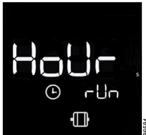
Figure 35: Running hours screen
