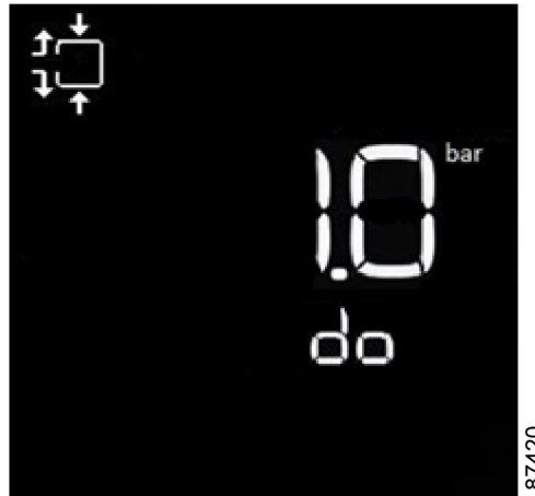
Figure 34: Direct stop level pressure changing
