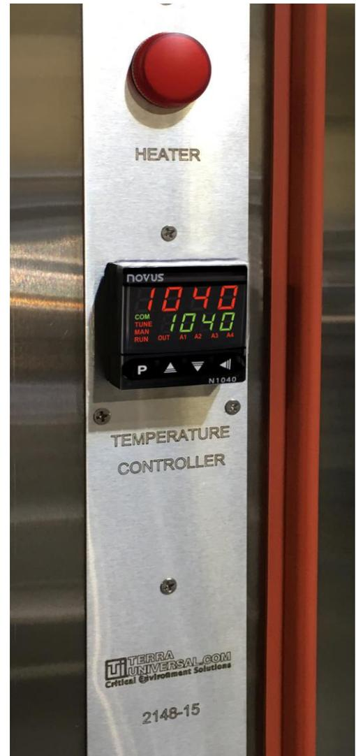
Figure 1. Temperature Controller
