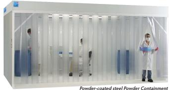
Powder-coated steel Powder Containment Room equipped with full-width strip shields
