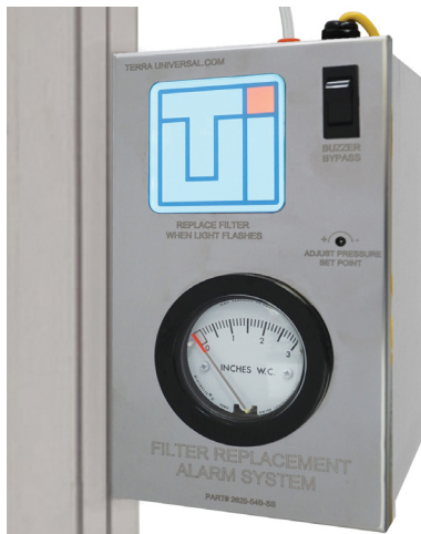
Cleanroom HEPA filter replacement alarm monitors backpressure and issues audible alert when filter requires replacement
