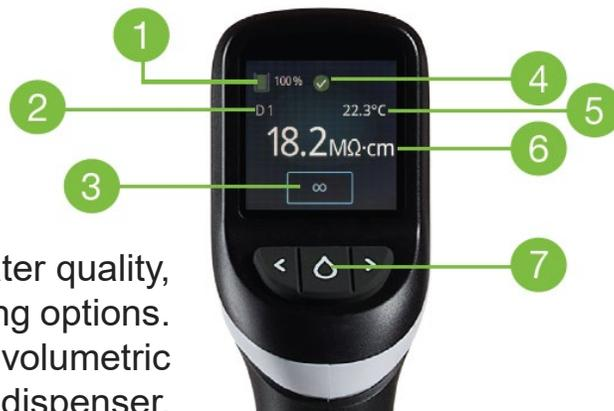
View key parameters like water quality, tank level, and dispensing options. Operate manual and volumetric dispenses right from the dispenser.
