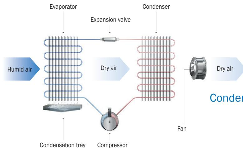
Condensation dehumidification — operating principle
