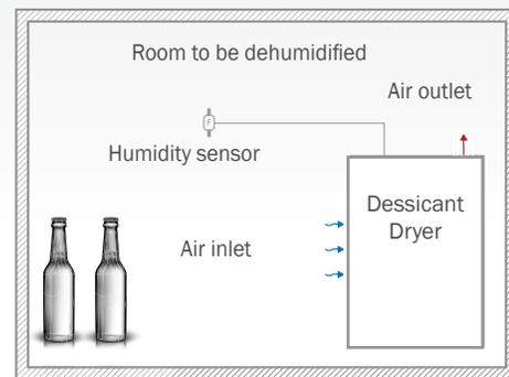
The figure shows a simple recirculation dehumidification process with a desiccant dryer. Heating modules, etc., can be configured and ensure a continuous supply of process air under the desired conditions and within the tolerances.
