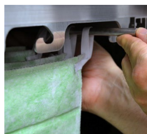
3 Place Support Rod on Hanging Supports
