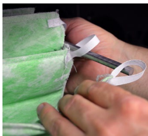
2 Thread Support Rod Through All Loops
