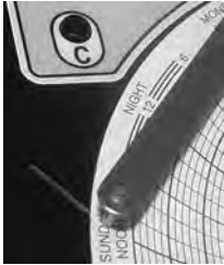
Chart recorder stylus and time line groove
