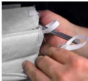
Thread Support Rod Through All Loops
