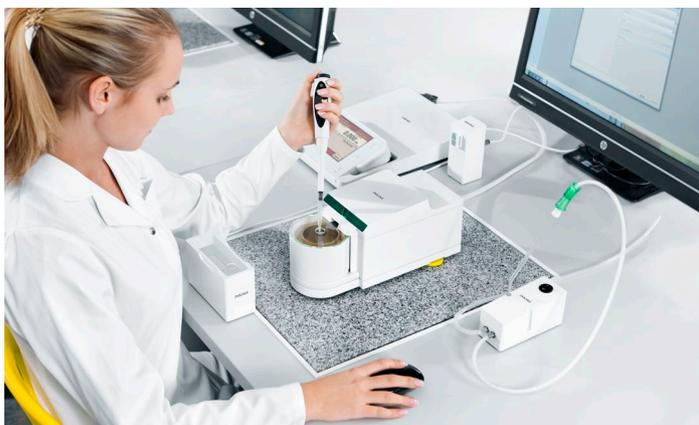
*For some electronic pipettes, such as Sartorius Picus® Nxt, the calibration interval can be set by activating the calibration reminder. The function will notify you when the previous calibration is about to expire. You can also lock the Sartorius Picus® Nxt pipette if you suspect that the pipette is not working properly; this prevents others from using the pipette until it has been checked.*
