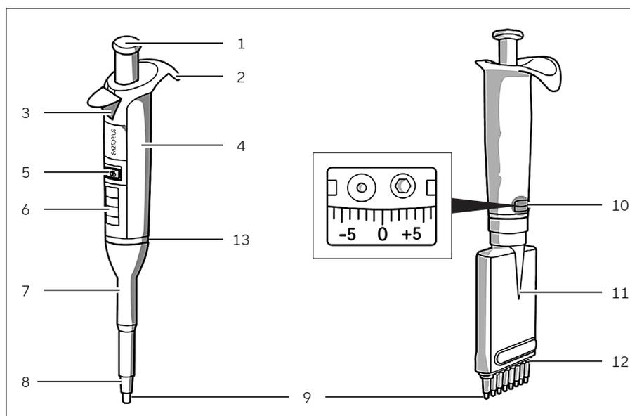
1. Operating button (polyamide (PA), silicone (SI), stainless steel (SS))
