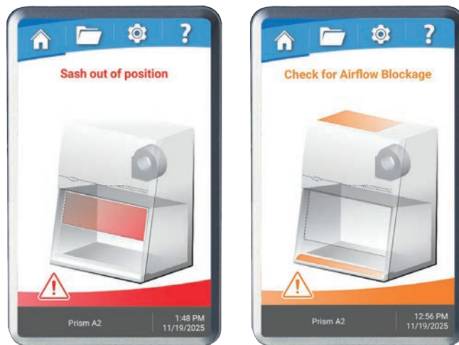
Sash Alarm and airflow blockage displays on Prism OS.
