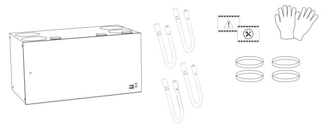
The installation kit includes: a UV caution decal, a maintenance decal, a pair of cotton gloves, a pair of 8" inlet collars, a pair of 8" outlet collars, Phillips screws (12) and larger screws for installation (4).
