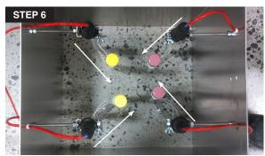
6. UV Lamp(s) and Ballast Position: The lamp should be positioned towards a central point in the middle of the unit's aluminum reflection chamber. For models with multiple lamps, you must position the lamps in a 'X' to bring them closer to the middle and optimize the UV dose of the unit.
