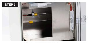
3. While holding the new UV lamp by its porcelain end-cap, slide it into the metallic reflection chamber.
