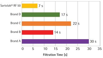
Comparison of filtration times for 50 mL cell media + 10 % FBS in five 0.22  $\mu m$  50 mL vacuum filtration units
