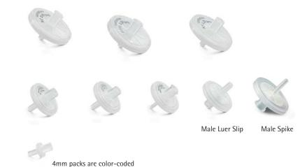
\* Sterile Minisarts are individually packaged. If not stated otherwise, Minisarts have been sterilized by ethylene oxide. The following Minisarts are NOT presterilized unless specifically noted. RC, PTFE and Nylon can be sterilized by autoclaving at 121°C for 30 min/or by using ethylene oxide (EO).
