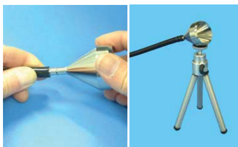
Figure 3-9 Tubing, Isokinetic Probe and Tripod
