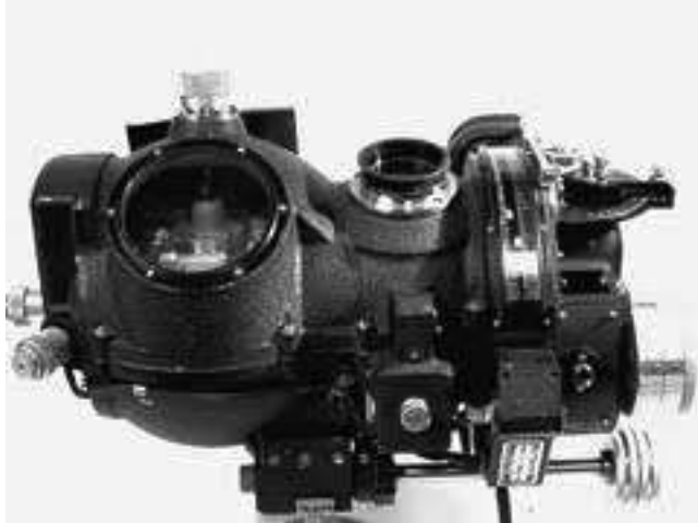
Figure 2. The Norden bombsight was designed in the 1930s, and went on to be used by most bombers in the U.S. Army Air Force during World War II. It was a complex analog computer, requiring unprecedented precision manufacturing. This drove the development of early cleanroom facilities and cleanroom techniques for micro-manufacturing.
